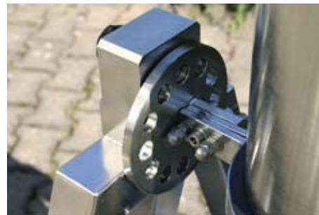
Notched wheels to fix a rotating column body.
